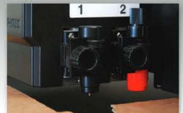
Dual Tool Holder for Cutting & Creasing (FC4510-60 Model)
